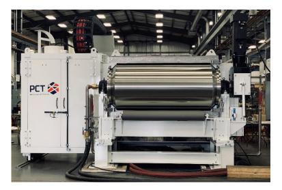
The Invictus series ebeam systems are the workhorses of ebeam processing equipment and are used for more demanding, high power applications. With accelerating voltages of up to 300 kV, these systems have the capacity to take on challenging applications. Need to crosslink multi-layer films, cure thick opaque coatings or process PSAs? Invictus is the proven answer for reliable performance.
