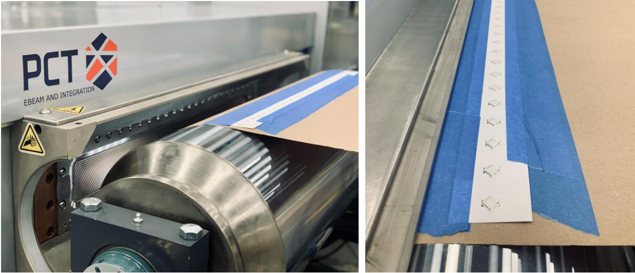
Figure 2. Dosimeter strips securely taped to a paper web with the dosimeters facing upwards.
