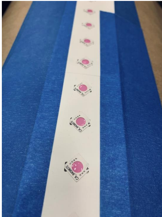
Figure 4. Dosimeters should change color to a shade of pink after being exposed to the ebeam (though not necessarily to the exact shade in this photo).
